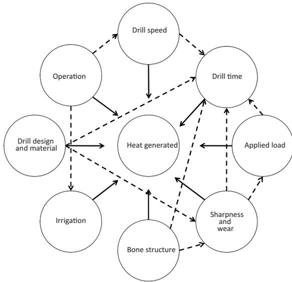
Fig. 2. Factors that interact during drilling of the implant site.
